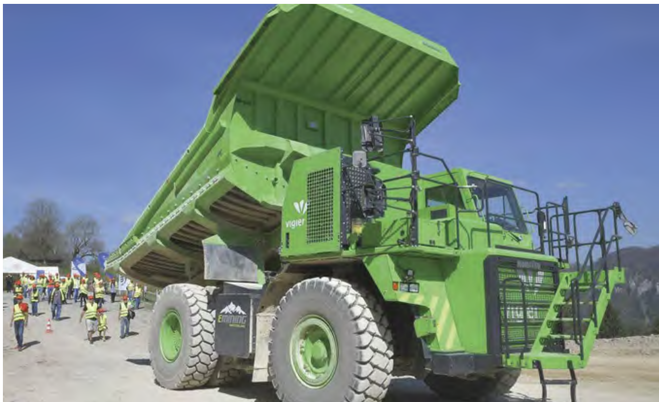
This eDumper runs on 700kWh batteries and regenerates excess energy to the power grid.
