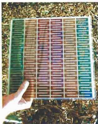
Various colours can be seen in a series-connected dye-sensitised solar cell (inset) (Image: Dr Winfried Hofmann RWE-Schott)
