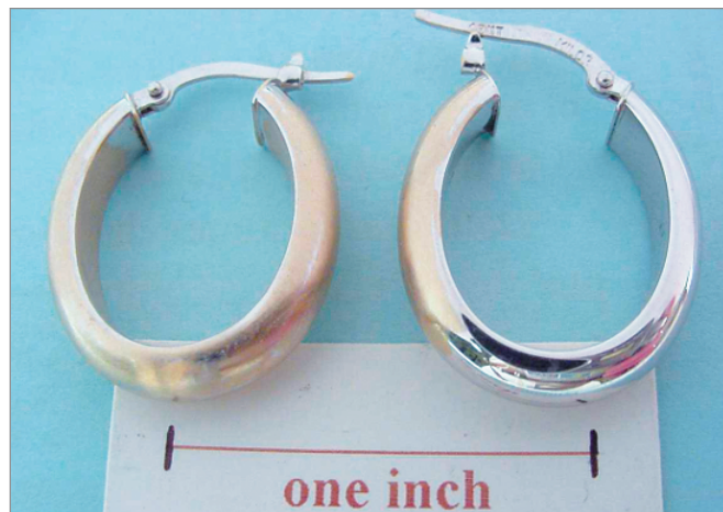
Figure 1 Example of a white gold earring with the rhodium plating removed to reveal the poor colour of the underlying 'white' gold (photo courtesy Stern-Leach)
