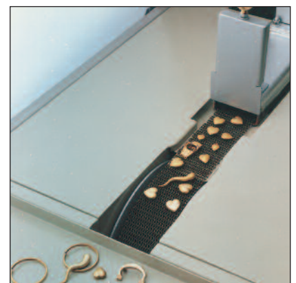
Figure 4.11 Soldering of stamped jewellery on a conveyor belt in a continuous furnace. (Courtesy IECO srl)
