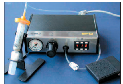
Figure 5.6 An electro-pneumatic solder paste dispenser. (Courtesy Hilderbrand & Cie SA)
