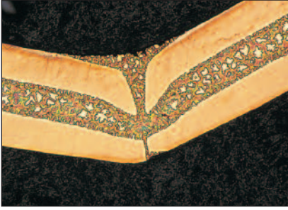
Figure 5.4a Photograph of a cross-section of a 14 carat gold chain link joined using solder-filled wire. a) A good joint
