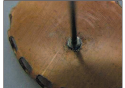
Figure 7.11 A typical electric discharge fusion weld. (Courtesy J. Alves)
