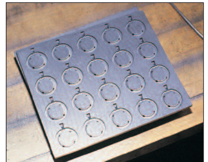
Figure 4.5a A CNC machined carbon board and paste solder
