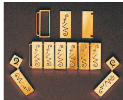
Figure 7.18 Parts of an 18 ct gold bracelet and earring set assembled by diffusion soldering at 450^{\circ}\text{C}
