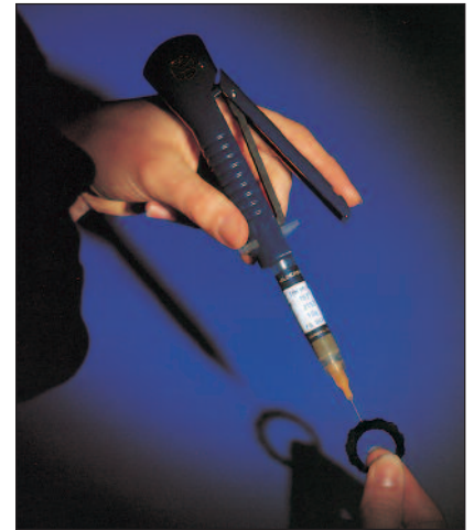
Figure 5.5b A hand-held solder paste dispenser in use. (Courtesy Hilderbrand & Cie SA)
