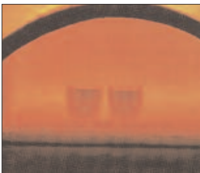
Figure 4. Samples in refractory cupels placed in furnace
