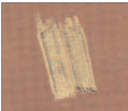
Figure 12. Rubbing from test piece (left) and touch needle
