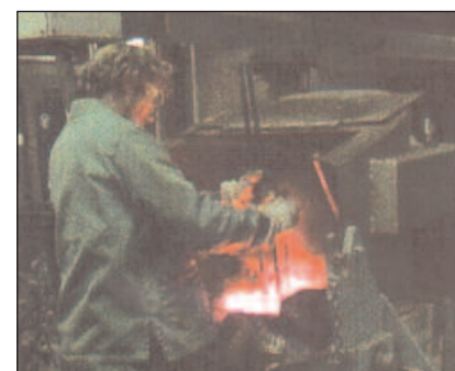
Sampling of molten bullion, to determine degree of fineness.
