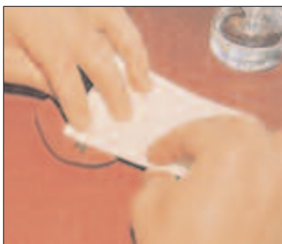
Figure 14. Soaking up excess acid with filter paper
