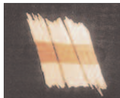
Figure 16. Rubbings of alloys containing 700 (left), 720 and 750 (right) parts per thousand gold
