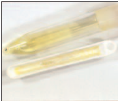
Figure 11. Centrifuge tube with cyanide solution (top) and ceramic boat after sample dissolution showing residual iridium (bottom)
