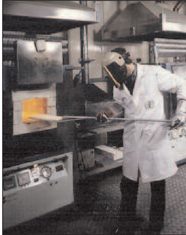
Fire Assay: Loading a cupel tray into the furnace
