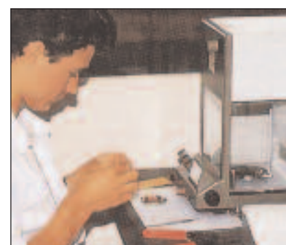
Figure 2. Weighing sample on an analytical balance
