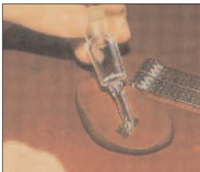
Figure 13. Applying touch acid to rubbings
