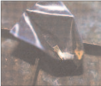
Figure 3. Wrapping gold sample and silver addition in lead foil
