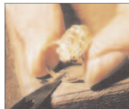
Figure 1. Sampling a gold ring by scraping
