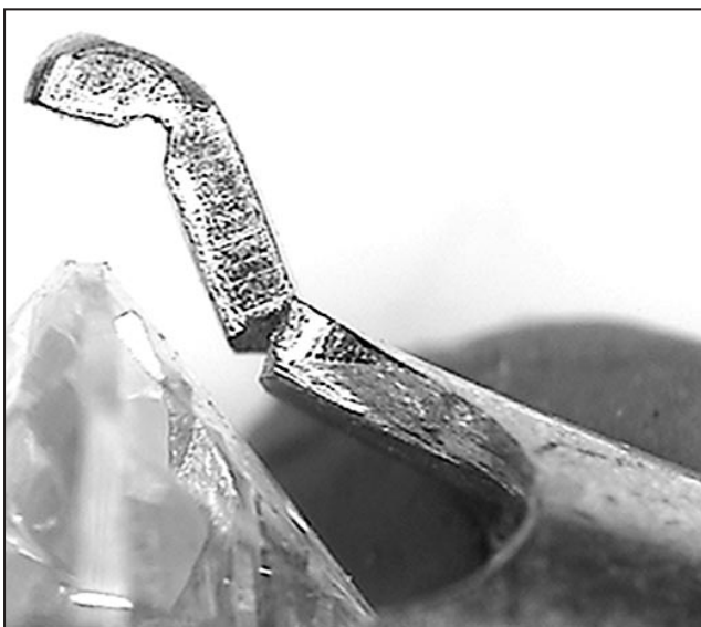
Figure 5 - A failed prong with stone still in place, 14ct nickel white gold
