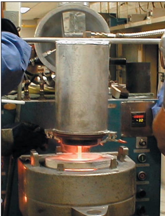
Figure 3 - Counter-gravity mould filling of an investment casting mould by a vacuum technique
