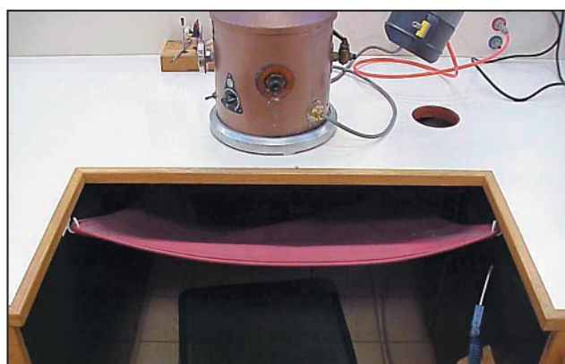
Figure 12 - Scrap wax capture with apron
