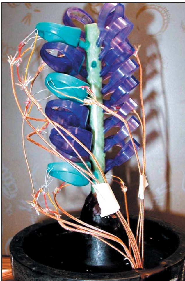
Figure 2 - Tree pattern with thermocouple attachments
