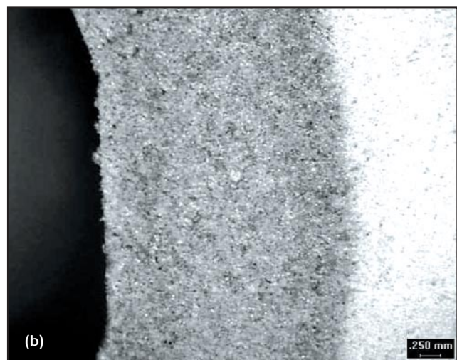
Figure 1 - Slit mould containing a wax pattern, removed from gas-fired burnout oven at start of 730°C/1350°F dwell. (a) Entire mould (b) Close up of wax penetration into investment
