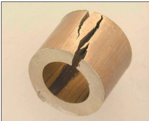
Figure 7 - Fire cracking in nickel white gold
