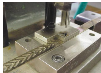
Figure 10 - The finished six-prong setting blanking tool mounted in a die set and shown in operation
