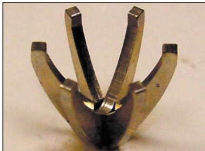
Figure 2 - A typical six-prong setting. Note the lack of solder in the joint allows a view of the interlock of the notches that hold the setting together
