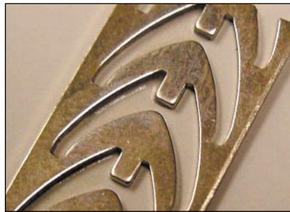
Figure 3 - Efficient use of material due to close nesting of the blanks on the strip
