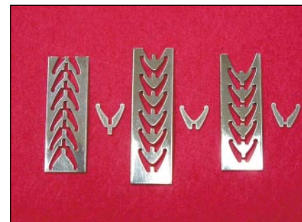
Figure 11 - The three blanks needed to assemble the six-prong setting and the scrap strips for each
