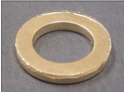
Figure 6 - This wedding band blank is a good example of improper gap between punch and plate. Note the large burr along the back edge
