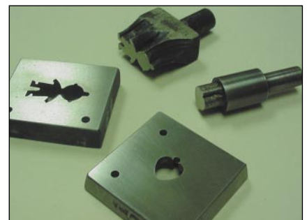
Figure 7 - Typical handmade charm blanking tools. They use the press stripper to remove the scrap material
