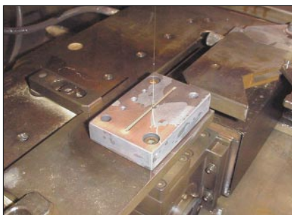
Figure 9 - The tools are cut with a wire EDM machine to a tolerance of .0002" (0.005mm)
