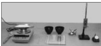
Figure 1 - A) Investment and scale, B) Thermometer, C) Rubber Bowls, D) Slump Ring, E) Mixing Head, F) Vicat, G) Timer
