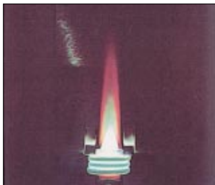
Figure 15 - Plasma flame in ICP Spectrometry (from reference 10)
