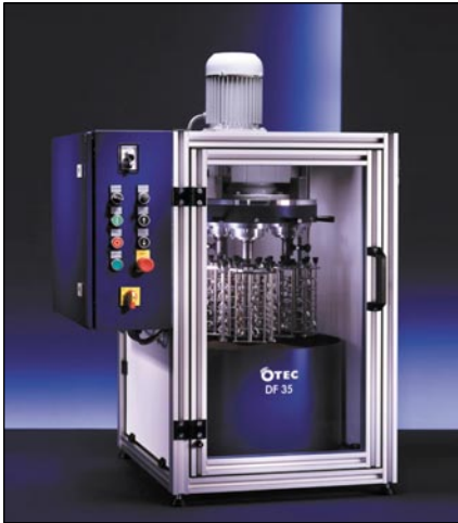
Figure 11 - Drag finishing machine (jewellery holder raised from container)
