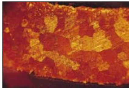
Figure 3 – Grain size of as cast PureGold
