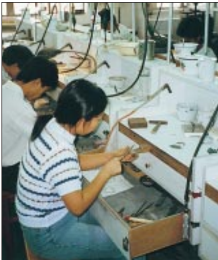
Figure 1 - Collection of dusts from workbenches should be part of a daily routine.
