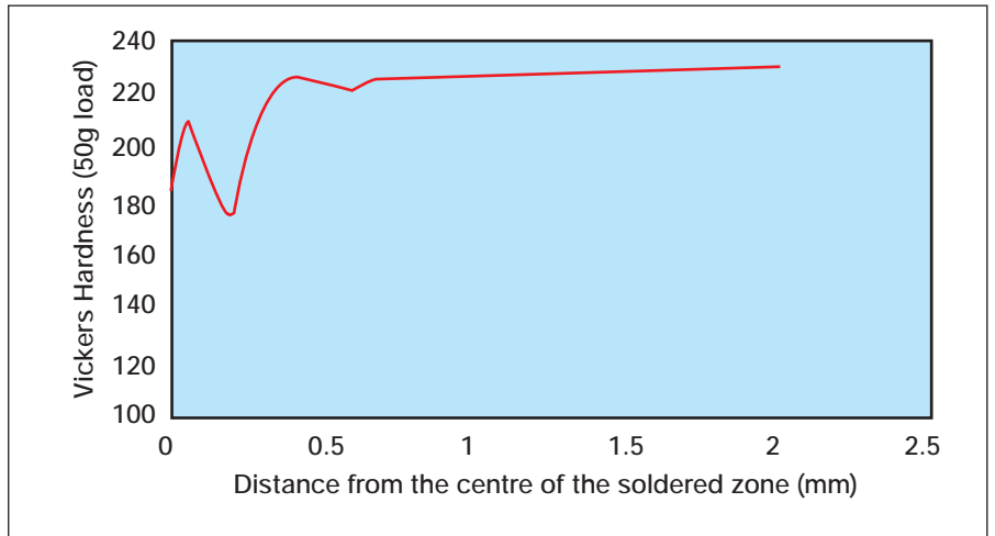
Figure 5 - Hardness profile of a soldered joint of hard 22-carat gold
