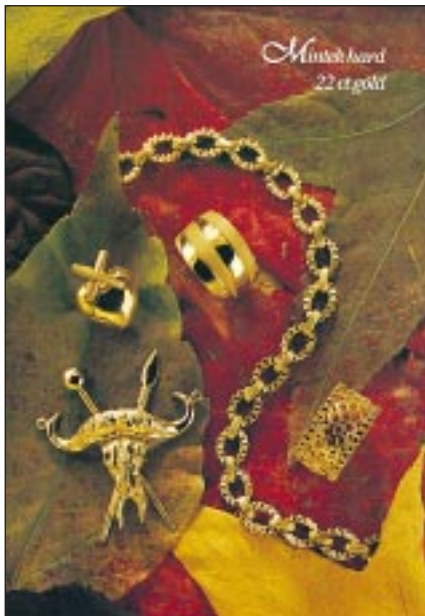
Figure 1a - Jewellery made of Mintek's hard 22-carat gold alloy by investment casting in air
