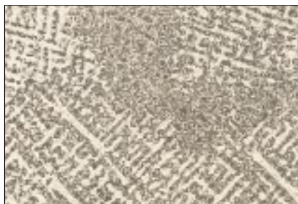
Figure 22 - Cast sterling silver showing non-equilibrium microstructure of primary \alpha surrounded by some eutectic \alpha + \beta
