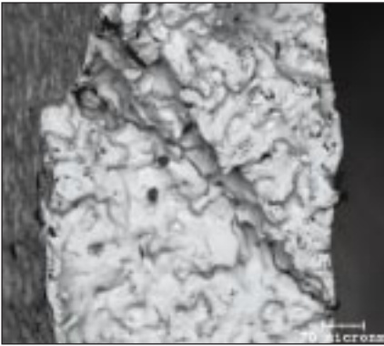
Figure 8 – Phase B on crack face
