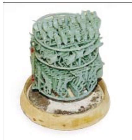
Figure 9 - Platform mounting of waxes on sprue
