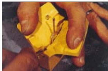
Figure 5 - Cutting the rubber mould
