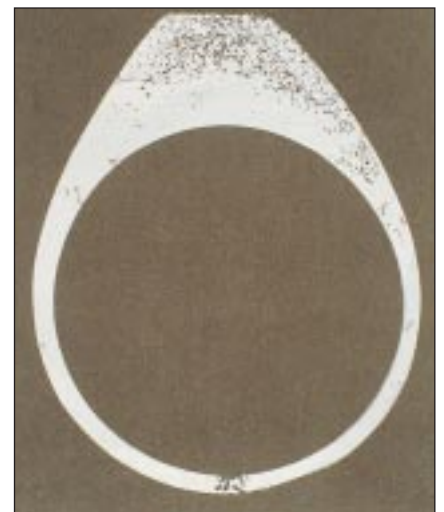
Figure 2 - Shrinkage porosity in 18 ct gold ring
