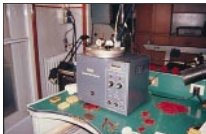
Figure 7 - Wax vacuum injector
