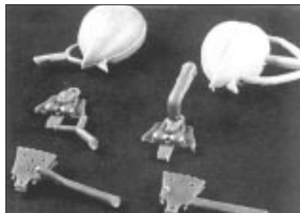
Figure 3 - Gating of wax patterns. (a) Left: as designed (b) Right: As modified for successful casting
