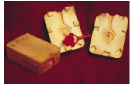
Figure 6 - Mould using prelocating pegs
