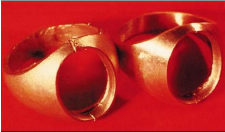
Figure 7 - Two castings of a signet ring. Left: the raw casting with pronounced parting lines and other imperfections which cannot be removed in the tumbling process; Right: a similar casting after being "cleaned up" by hand before the cutting cycle.
