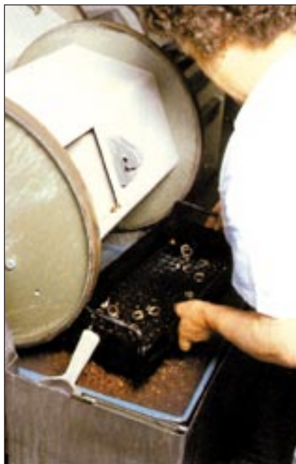
Figure 1 - Barrel finishing. The operator is separating parts from media after the cutting cycle.
