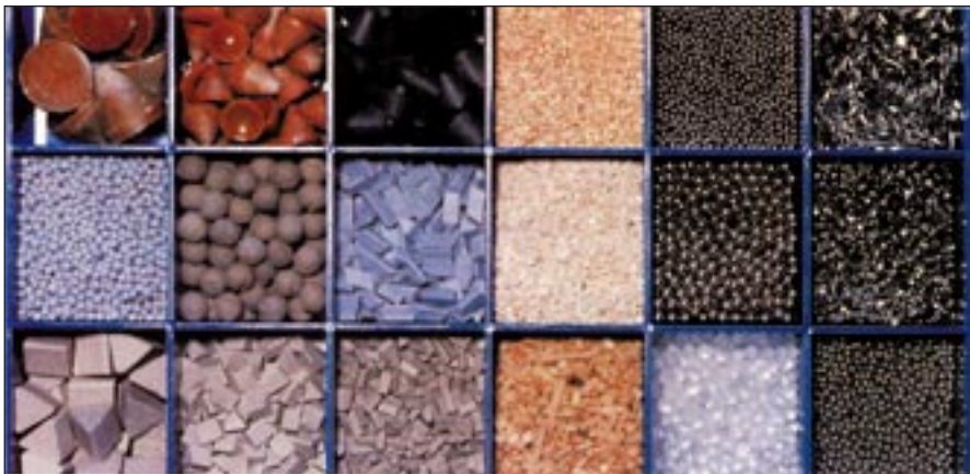
Figure 6 - A selection of media used in barrel finishing processes.
