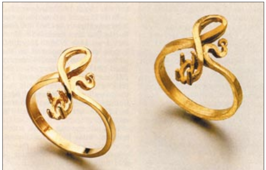
Figure 8 - Before and after... This photograph of two gold rings gives a good indication of what can be accomplished with modern tumbling processes.
