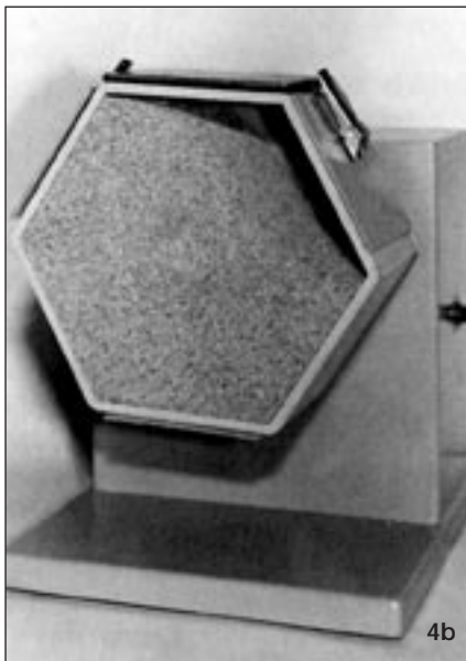
Figure 4a-b - The effect of filling ratio on the slide zone in a barrel rotating at the optimum speed.
