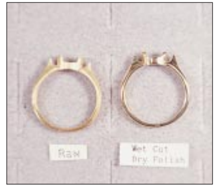
Figure 1 - Cast 18 carat gold ring: On the left is the as cast ring with gate cut off and ground; on the right is same ring after a three step finishing process in a vibratory machine
