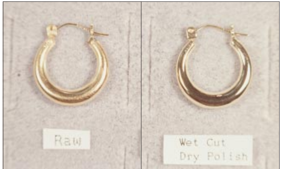
Figure 3 - Thin wall gold earring: (a) Finding after soldering operation (b) After two step vibratory finishing.
