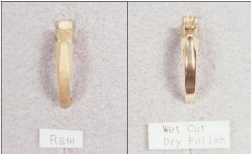
Figure 2 - Magnified side view of ring in Figure 1. (a) As cast (b) After vibratory finishing
