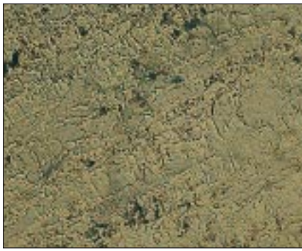
Figure 2 - OB-18 alloy before annealing (x 500)
