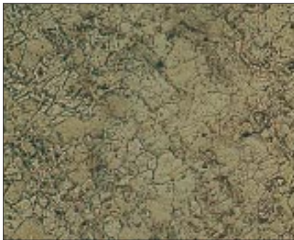
Figure 3 - OB-18 R alloy after annealing
