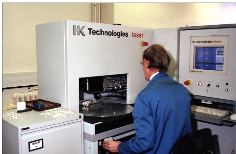
Figure 1 - The laser marking equipment
