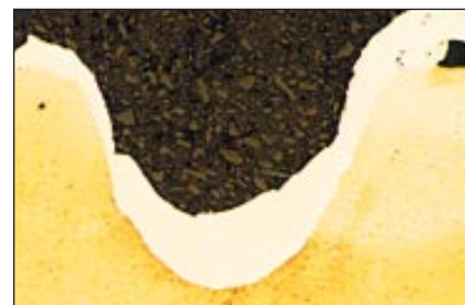
Figure 2 - Platinum powder melted into a gold substrate with too high a laser intensity
