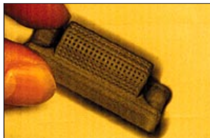
Figure 6 - Rapid Prototyping by laser sintering
