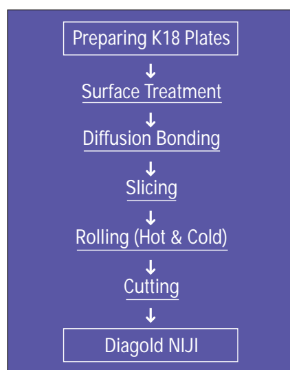
Figure 2 - The production of Diagold - schematic
