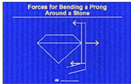
Figure 2 - Forces involved in bending a prong around a gemstone (schematic)
