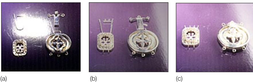
Figure 7 - Two cast 14 ct gold pendants with cast safety catches: (a) the separate components, (b) the safety catches hooked onto the pendants, (c) the safety catches pushed into the locked position (Courtesy of Anthony Eccles)
