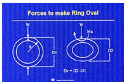
Figure 8 - Force to make a ring oval (schematic)
