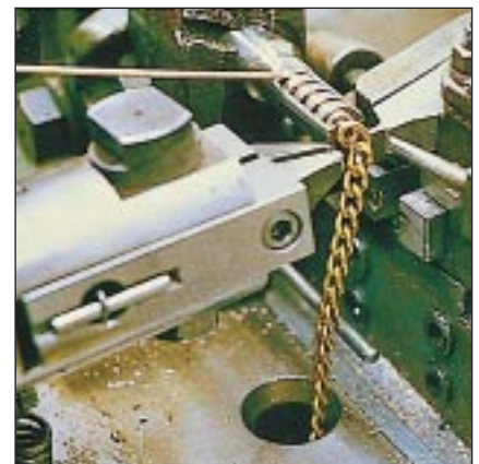
Figure 10 - Chain making involves bending and twisting of wire
