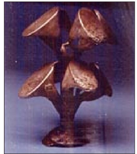
Figure 14 - Defects in cast rings that can be ascribed to excessive pressure during centrifugal casting
