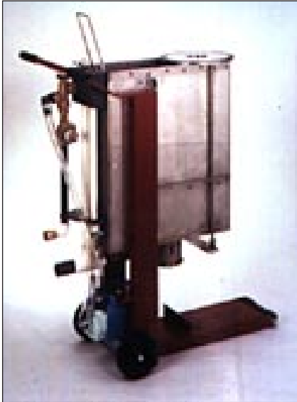
Figure 12 - Graining attachment for making alloy grains of the required caratage and homogeneity
