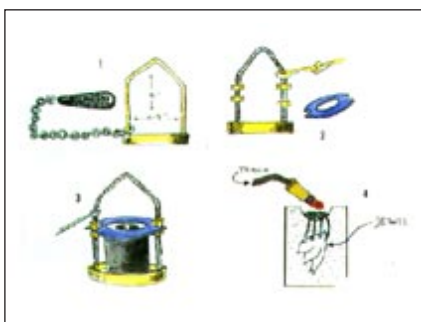
Figure 1 - a) Preparation of the flask and of the sling caster; torch melting in the dome-shaped opening at the mouth of the flask.
