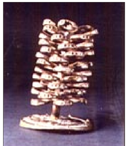
Figure 15 - Incomplete filling of centrifugally cast items (on the right side of the tree)
