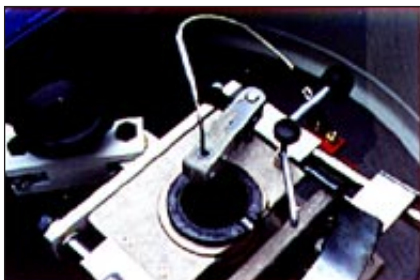
Figure 4 - Detail of a variable geometry centrifugal casting machine with the temperature measurement attachment (dipping thermocouple)
