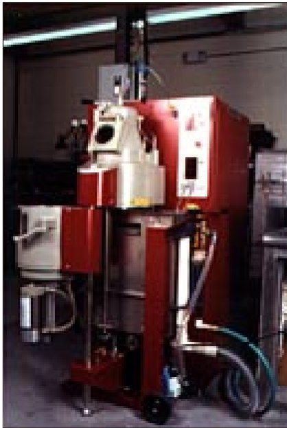
Figure 13 - Casting equipment with the grainer in position, in place of the mould chamber
